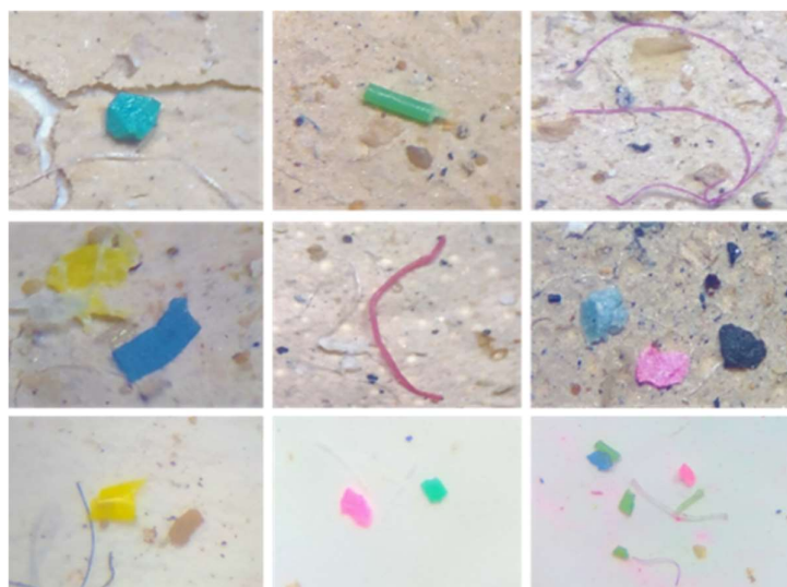
Figure 4. Determination of microplastics in sediments under fluorescence microscopy.
